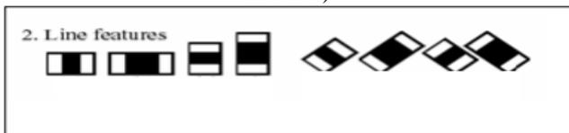
Figure 10: A set of extended Haar like Feature (Line features)
