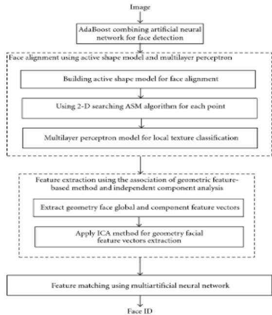
Figure 13: Proposed models for steps of a face recognition system.
