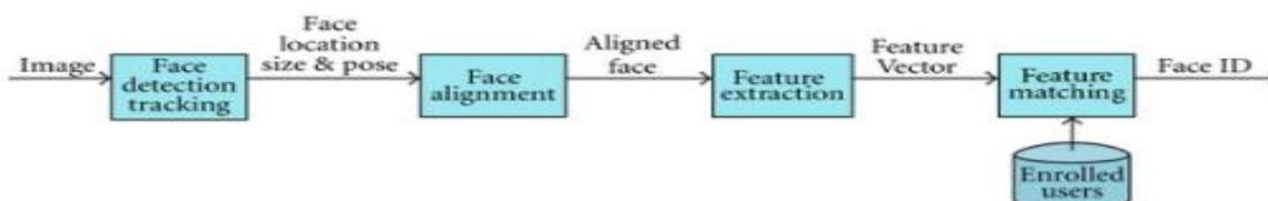
Figure 1: Structure of a face recognition system
