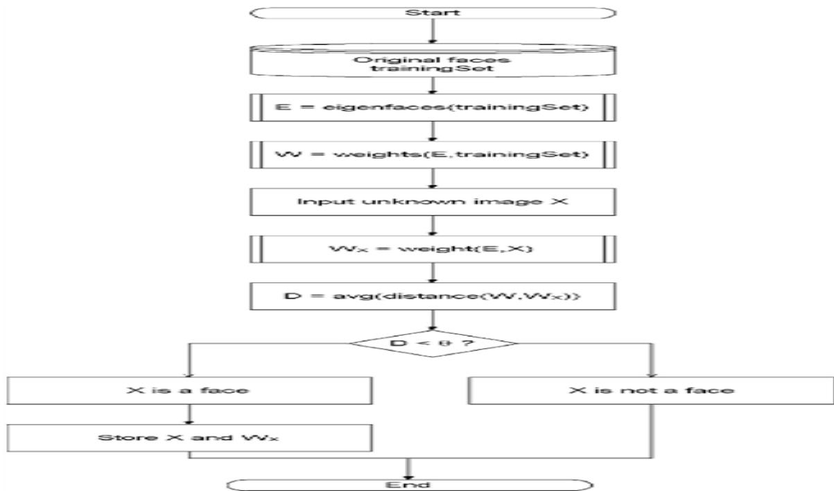
Figure 14: Flow chart of the Eigen face-based algorithm
