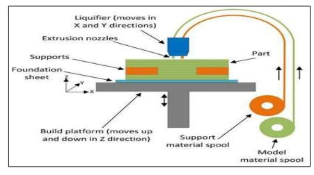
Figure.1. Fused deposition modeling (FDM) setup [4]
