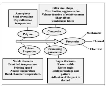
Fig.2 Various parameters influencing the properties of FDM printed parts [28]
