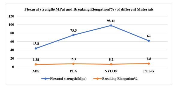
Figure.5 Flexural strength (MPa) and Breaking Elongation (%) of some materials [35]
