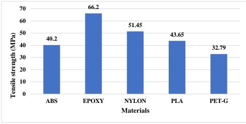
reinforced silicon carbide, EPOXY and NYLON have higher tensile strength than ABS and PLA (Cf-SiC).
