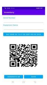
Opening the QR Code Scanner, scans the QR Code which is attached to each item and after the QR Code is scanned the item related information will be shown on the screen which contains the product description, Serial No of the product, Date of installation, previous maintenance record and updated record.
