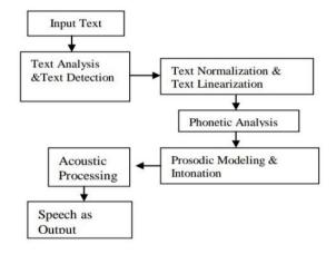
Figure 4. Block diagram of TTS
