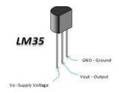
Fig 6: LM35 thermistor with pin configuration
