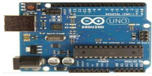
Fig 4: Arduino uno micro-controller
