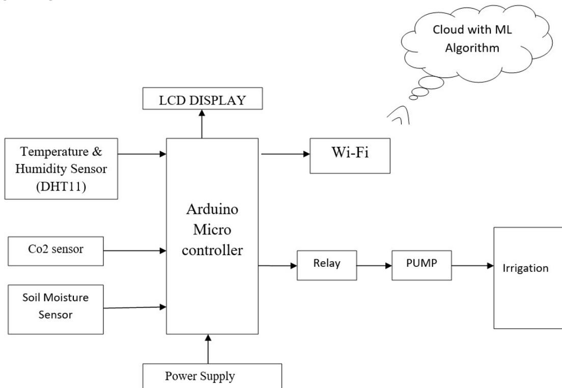
**Fig (1) using micro controller drip irrigation overview**
