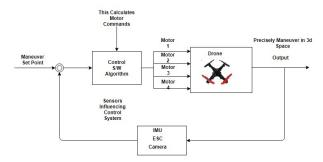
Figure 3. Control Parameters of the drone
