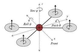
Figure 2. Control Parameters of the drone
