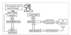
Figure 1: Block Diagram of ViTel
