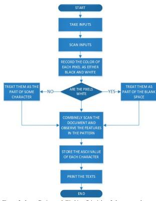
Figure 3. Inner Design and Working Principle of the proposed scanning application
