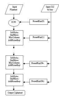
Figure 1. Encryption procedure of AES 512
