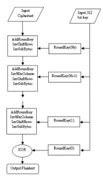
Figure 2.procedure of AES 512
