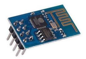
Figure 5. ESP8266 Wi-Fi Wireless Transceiver module
