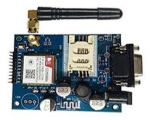
Figure 7. SIM800A GSM Board
