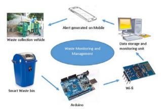
Figure 1. Schematic diagram of Waste monitoring and management solution
