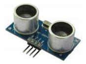
Figure 2. Ultrasonic sensor module: HC-SR04
