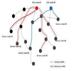
Fig 1: Multi-rate multicast wireless sensor network
