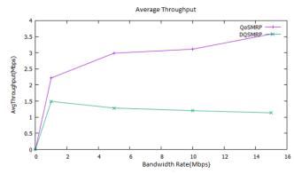
Fig 8: Average Throughput: Bandwidth Rate vs Throughput
