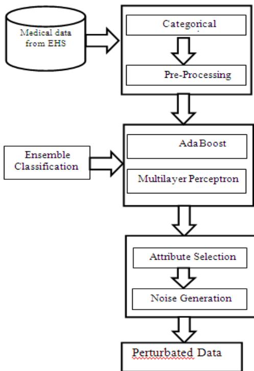
Figure 3.1: PPECH system Architecture
