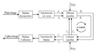
Figure 2. Block diagram of Image cryptosystem
