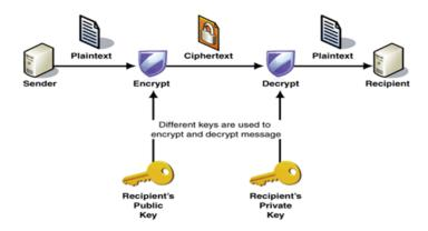
Figure 3: Asymmetric Key Encryption Process
