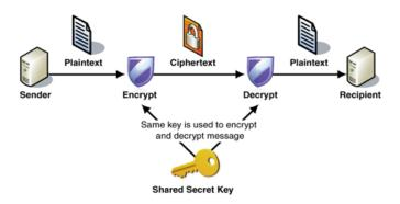
Figure 2: Symmetric Key Encryption Process
