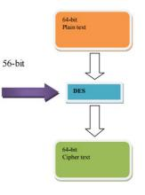
Figure 4: The conceptual working with DES
