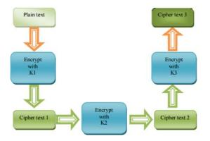
Figure 5: Encryption process Triple DES with three keys K1, K2 and K3
