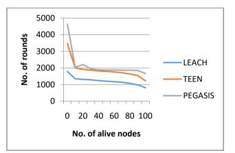
Fig3: Network Lifetime of Homogeneous WSN
