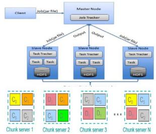
Figure No 2: Programming Model ofHadoop processing framework [4]
