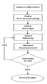
Fig. 3. Process of web data mining
