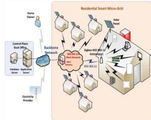
**Fig.4. Smart Micro-Grid AMI Architecture**
