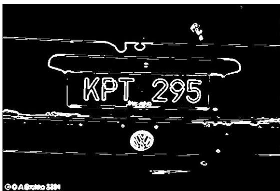
Figure 8 Image with eliminated possible horizontal lines
