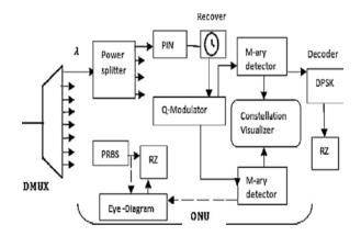
Figure 4: Schematic diagram of Optical Network Unit (ONU) in hybrid PON [10]
