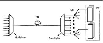
Figure 1: hybrid WDM TDM PON [10]
