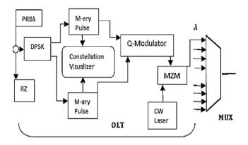
Figure 3: Schematic diagram of Optical Line Terminal (OLT) in hybrid PON [10]
