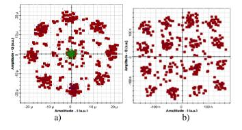
Figure 6: Constellation diagrams at receiver, for a) 8-DPSK, and b) 16-QAM
