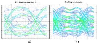
Figure 7: Eye diagrams at receiver for 5.1 Gbps data rate, for a) 8-DPSK, and b) 16-QAM
