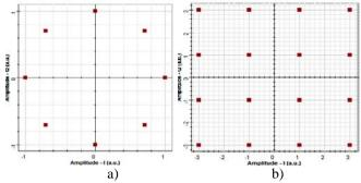
Figure 5: Ideal constellation diagrams at transmitter, for a) 8- DPSK, and b) 16-QAM
