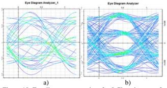
Figure 10: Eye diagrams at receiver for 8 Gbps data rate, for a) 8-DPSK, and b) 16-QAM
