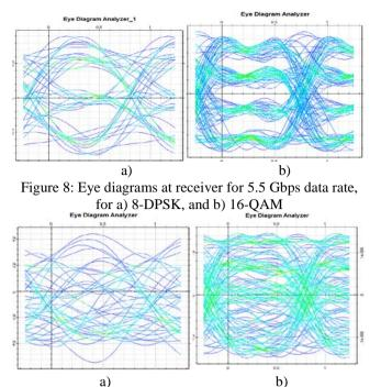
Figure 9: Eye diagrams at receiver for 6 Gbps data rate, for a) 8-DPSK, and b) 16-QAM
