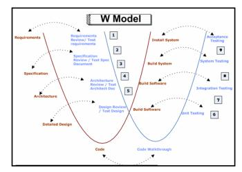
Figure 4: W Model where Each phase is verified/validated. Dotted arrow shoes that every phase in brown is validated/tested through every phase in sky blue.
