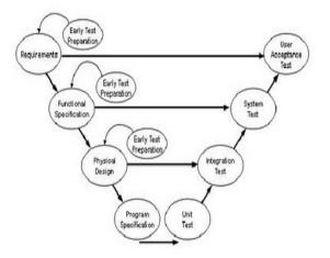
Figure 2: The V-Model with early test preparation.
