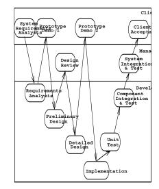
Figure 6: Shark tooth model with two prototype demonstrations
