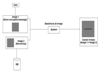
Fig. 1 DFD of how visual cryptography applied in the system
