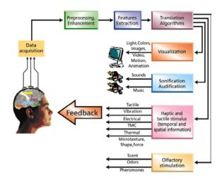
Figure3: Conceptual BCI system with various kinds of Neurofeedbacks[5]
