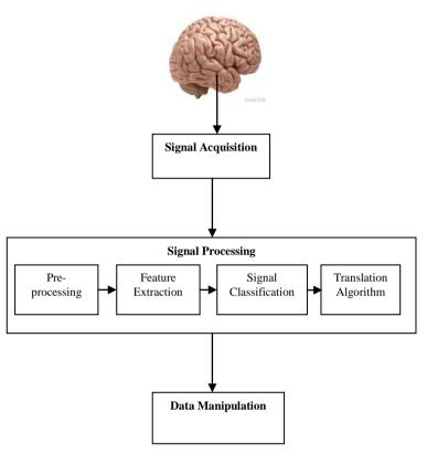
Figure2: BCI Signal Processing
