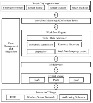
Figure 1.3.Cloud-based Workflow Architecture for Smart City
