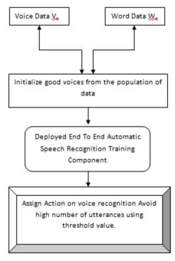
Then we are deploying the end to end automatic speech recognition training component. This training component helps to understand and execute the natural language into machine language for providing the proper guidance to the artificial intelligence. It can be make professional artificial intelligence neurons with the help of provided regular correct training data sets. The Re-estimation of voice
