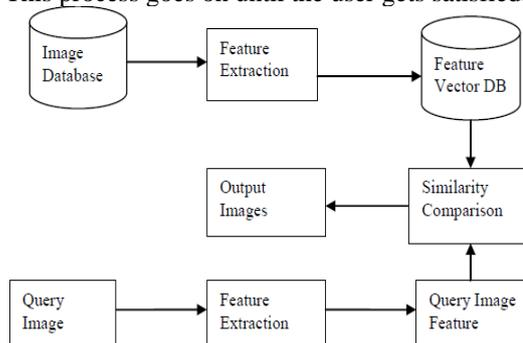
Fig 3: Block Diagram for CBIR Technique
