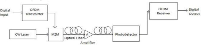
Fig.3.1 Block diagram of OOFDM-ROF system. [11]
