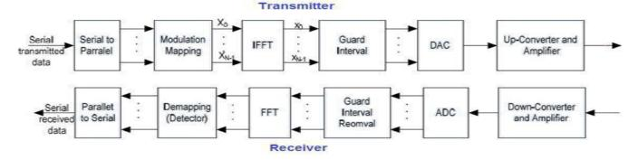
Fig.1.1 OFDM (orthogonal frequency division multiplexing). [19]
