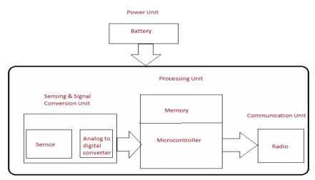
Fig1.1 A typical sensor node structure
