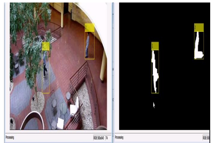
Figure.5: Human motion detection/ Video detections using wavelet threshold Motion detector
