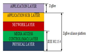
Fig 1: ZigBee protocol stack
