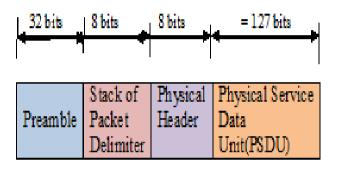
Fig 2: IEEE 802.15.4 Physical layer packet structure
