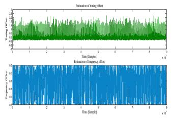
Figure 8. Peak values (Top) gives the timing estimation indices. At these time instants (Bottom) give the Frequency offset estimation in AWGN channel
