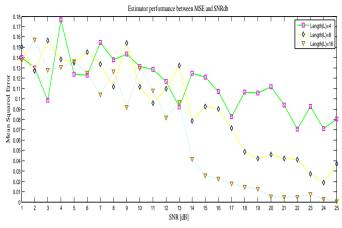
Figure 7. Performance of Frequency Estimators for the random noise channel (L=4, L=8 and L=16) as the function of Mean square error with SNR.
