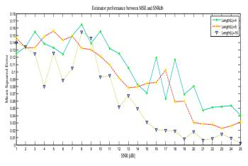
Figure 10. Performance of Frequency Estimators for the AWGN channel (L=4, L=8, and L=16) as the function of Mean square error with SNR
