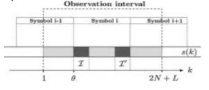
Figure 2. Structure of OFDM signal with cyclically extended symbols s (k), the Set I contain the cyclic prefix, i.e., the copies of the L data samples in I :
