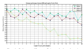
Figure 6. Performance of Frequency Estimators for the random noise channel (5, 10, and 15 dB) as the function of Mean square error and Cyclic prefix Length (1 to 20 samples).
