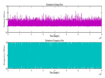
Figure 5. Peak values (Top) gives the timing estimation indices. At these time instants (Bottom) give the Frequency offset estimation in Random Noise channel.
