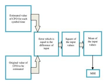
Figure 4. Block diagram for calculating MSE of the estimator
