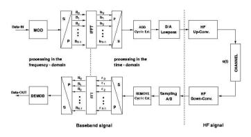
Figure 1. Basic OFDM system model
