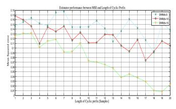
Figure 9. Performance of Frequency Estimators for the AWGN channel (5, 10, and 15 dB) as the function of Mean square error and Cyclic prefix Length (1 to 20 samples).
