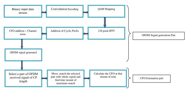
Figure 3. Block diagram of ML technique using CP based estimator
