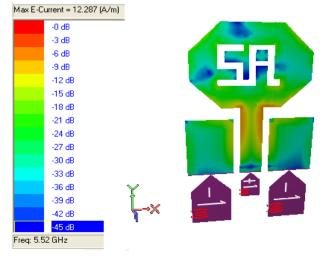
Figure 8: Current distribution of proposed Antenna at 5.52 GHz
