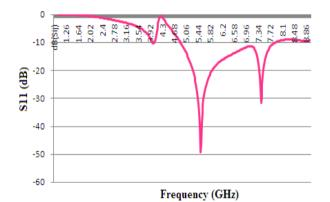
Figure 2: Return losses of proposed antenna
