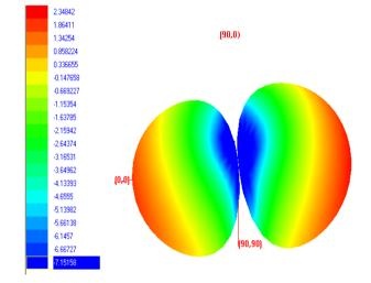
Figure 7: 3-Dimensional Pattern of Proposed Antenna at 5.52 GHz
