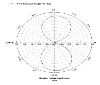
Figure 6(a): Elevation pattern at 5.52 GHz
