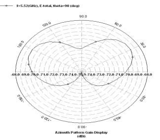
Figure 6(b): Azimuth pattern at 5.52 GHz
