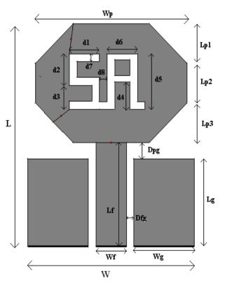
Figure 1: Geometry of proposed Antenna
