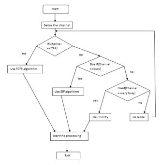
Figure 5: Flow Chart of Proposed Algorithm
