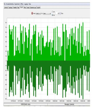
Figure 5 Graph when packet flooding attack is launched from Node D to Node C.
