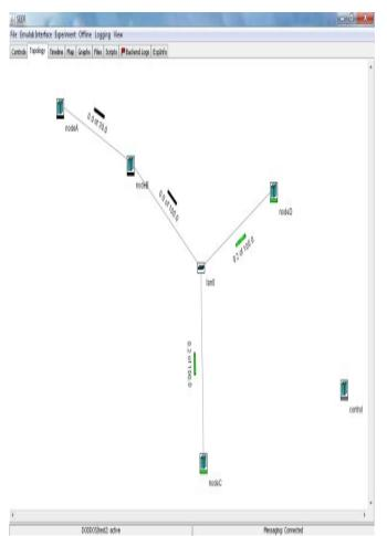
Figure 3. Experimental Topology in seer showing packet flooding attack from Node D to Node C.
