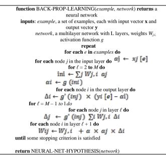
Figure 6. The back-propagation algorithm for learning in BPN networks
