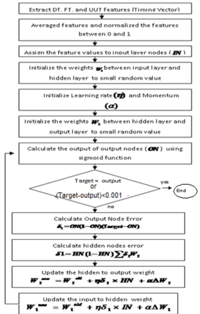
Figure 4: Keystroke Dynamics with Backpropagation Network
