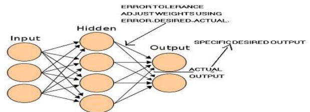
Figure 3: Structure of Backpropagation Network
