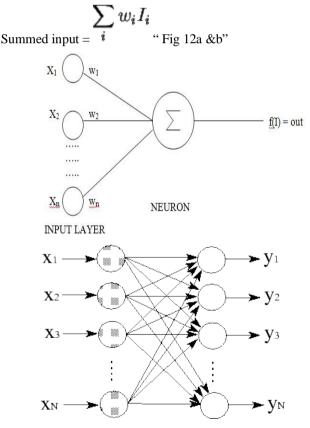
Figure 12. Single layer feed forward network
