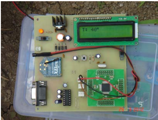
Figure.5 Temperature display on slave node photo
