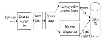
Figure.1 block diagram of the proposed system
